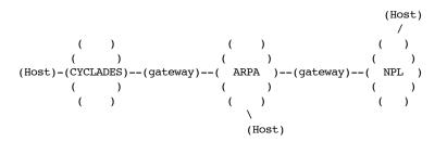
Also there was a diagram of data going from a host computer on one computer network to a gateway and then to a host on another computer network.
